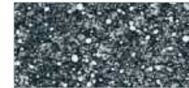
Pulvermetallurgischer HSS-Bohrer • feine Mikro-Kornstruktur • gleichmäßige Kornverteilung • höchste Festigkeit Powder metallurgy HSS-drills • fine micro grain structure • even grain formation • highest strength Struttura di HSS-PM • struttura a grani fine • struttura compatta e uniforme • massima resistenza
